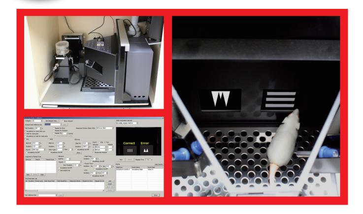
Visuals (both static image and animation) can be displayed through LCD panel and touch response recorded through the special application software. Based on the touch response, reward (pellet or liquid) can be provided.
