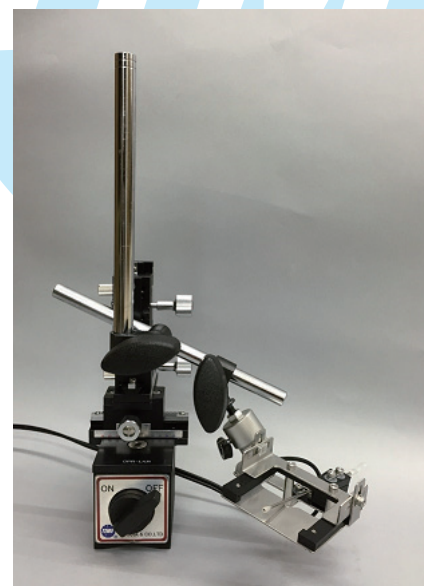
Licking sensor with XYZ manipulator
